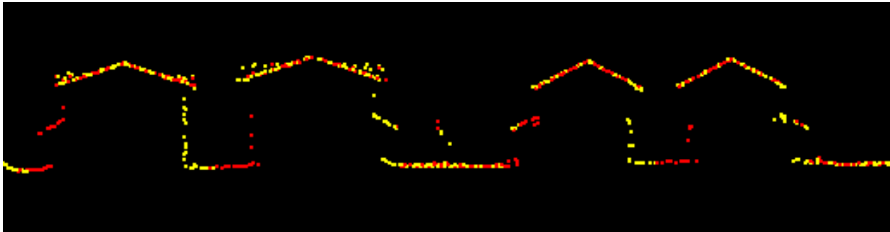
Figure 8– Horizontal Alignment. Two separate flight lines differentiated by color (Red/Green) are shown in this profile. There is no visible offset between these two flight lines. No horizontal alignment issues were identified.
