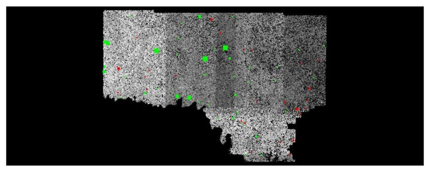
Green represents where the lidar surface is above the check point (positive elevation error).
