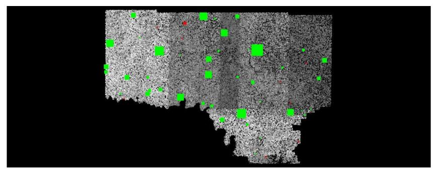
Green represents where a DEM of the lidar surface is above the check point (positive elevation error).
