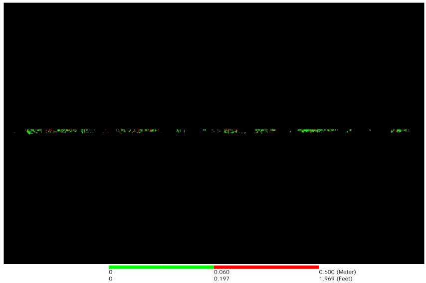
A maximum vertical separation cutoff has been applied to this graphic for the purpose of masking out disruptive features that are not applicable for depicting sensor noise within individual swaths (e.g., trees, moving cars, etc.).
