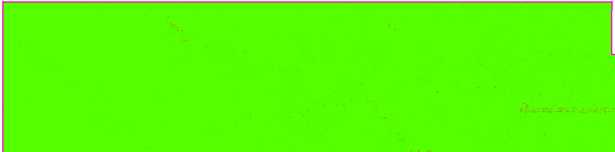
Figure 78– Spatial Distribution for Block 10. All cells (2*NPS cellsize) containing at least one lidar point are colored green. Cells that do not contain a lidar point, including water bodies which are acceptable NoData area, are colored red. Without removing acceptable NoData areas due to water, at least 98% of cells contain at least one lidar point.
