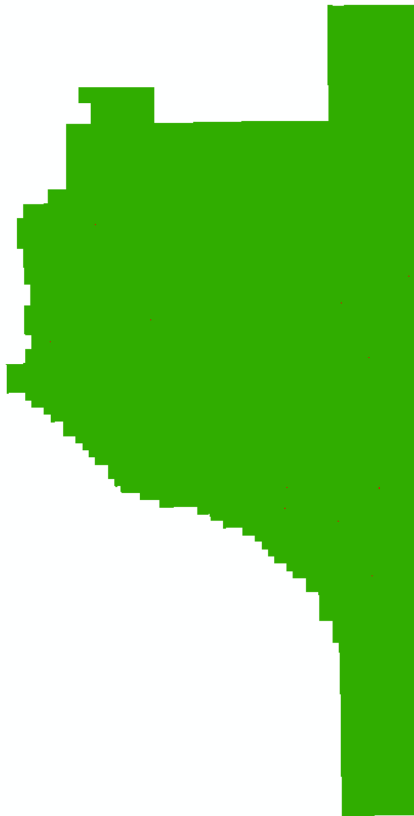
Figure 70– Spatial Distribution for Block 01. All cells (2*NPS cellsize) containing at least one lidar point are colored green. Cells that do not contain a lidar point, including water bodies which are acceptable NoData area, are colored red. Without removing acceptable NoData areas due to water, at least 98% of cells contain at least one lidar point.
