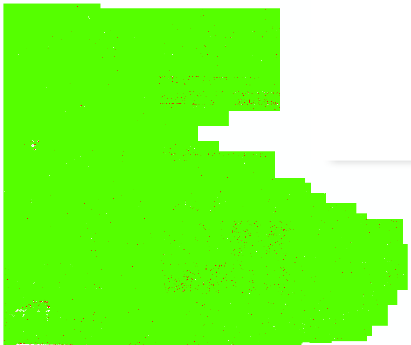
Figure 66– 1-square meter density grid for Block 12. There are some 1-meter cells that do not contain 2 points per square meter (red areas) due to the irregular spacing of lidar point cloud data. Most 1-sqaure meter cells contain at least 2 points per square meter (green areas) showing there are no systematic density issues. When density is viewed/analyzed by representative 1-square kilometer areas, density passes with no issues.
