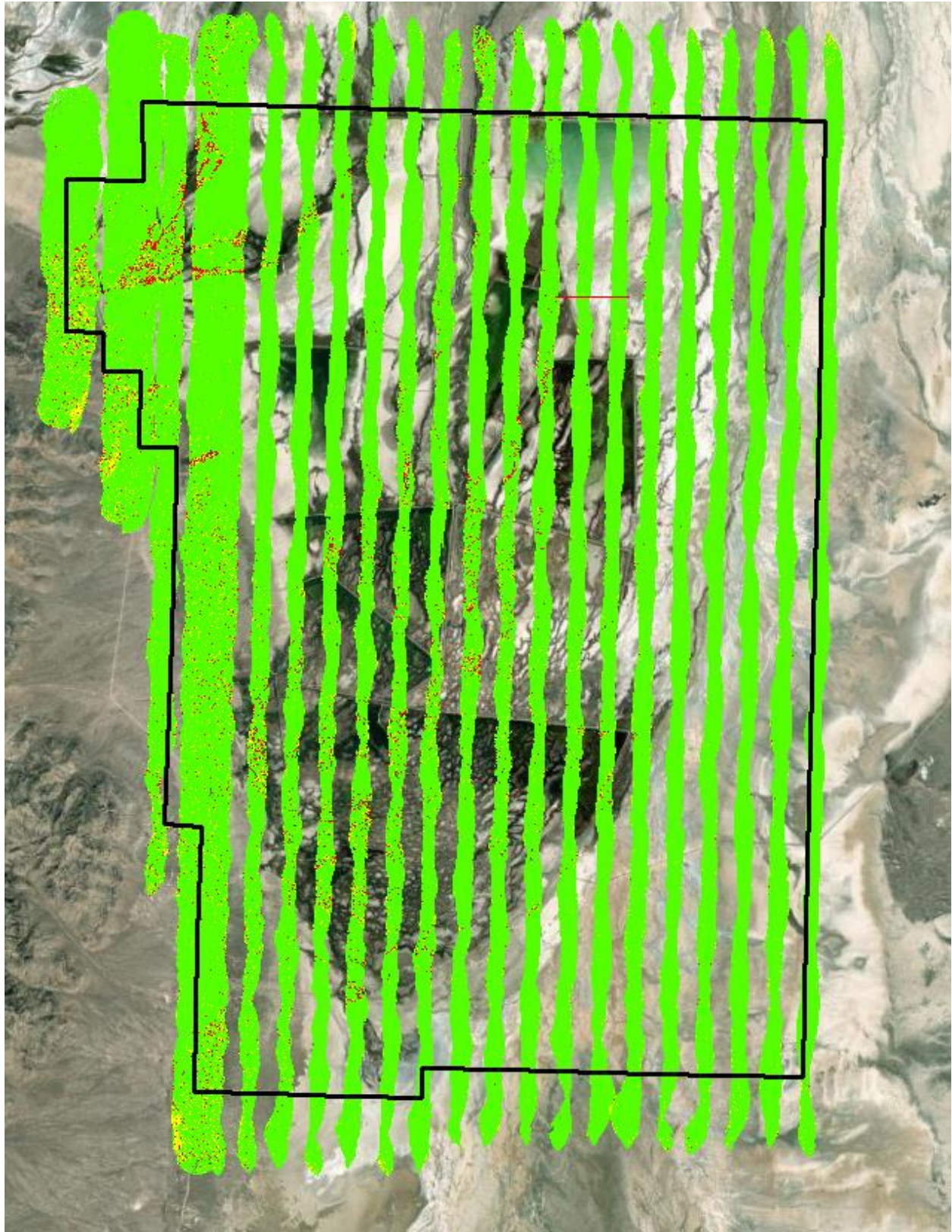
Figure 5. Single return interswath DZ rasters for the Fish Springs Topobathymetric Lidar Project.
