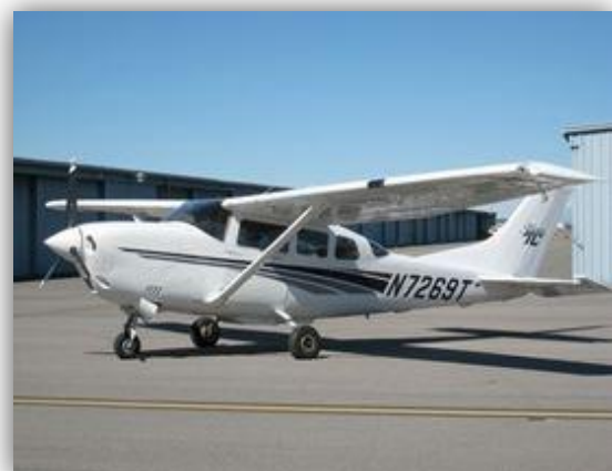
Exhibit 3: The acquisition platform for the Millsite Reservoir project was a turbocharged Cessna 206. Our 206 has been customized for LiDAR and other airborne sensors with an upgraded power system and avionics. The stability of the Cessna 206 is ideal for LiDAR collection
