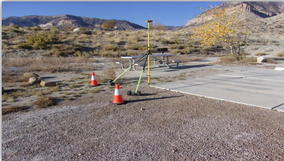
Exhibit 6: Calibration Control Point (Base)
