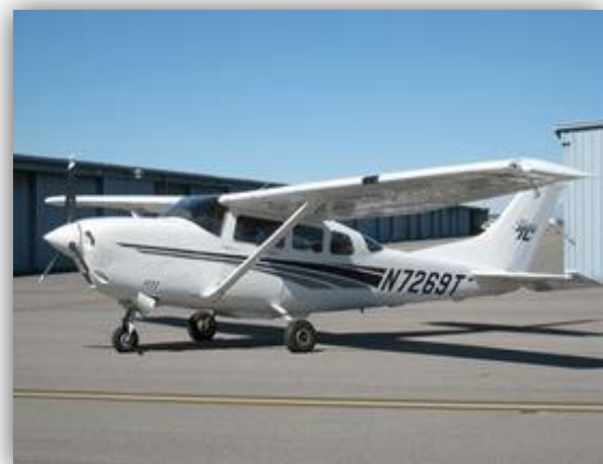
Exhibit 3: The acquisition platform for the Strawberry River project was a turbocharged Cessna 206. Our 206 has been customized for LiDAR and other airborne sensors with an upgraded power system and avionics. The stability of the Cessna 206 is ideal for LiDAR collection
