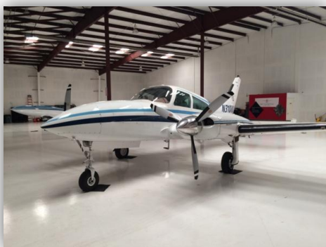
Exhibit 8: The imagery acquisition platform for the Strawberry River project was a turbocharged Cessna 310. Our 310 has been customized for imagery and other airborne sensors with an upgraded power system and avionics. The stability of the 310 is ideal for imagery collection.
