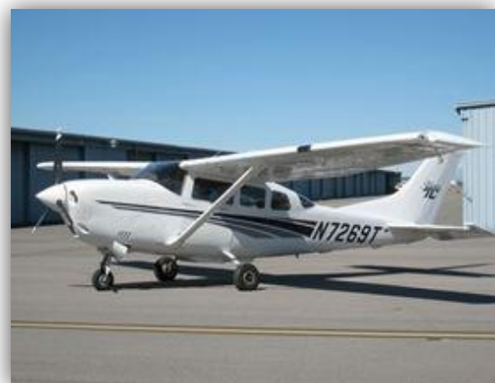
Exhibit 3: The acquisition platform for the Washakie & Whites Valley project was a turbocharged Cessna 206. Our 206 has been customized for LiDAR and other airborne sensors with an upgraded power system and avionics. The stability of the Cessna 206 is ideal for LiDAR collection
