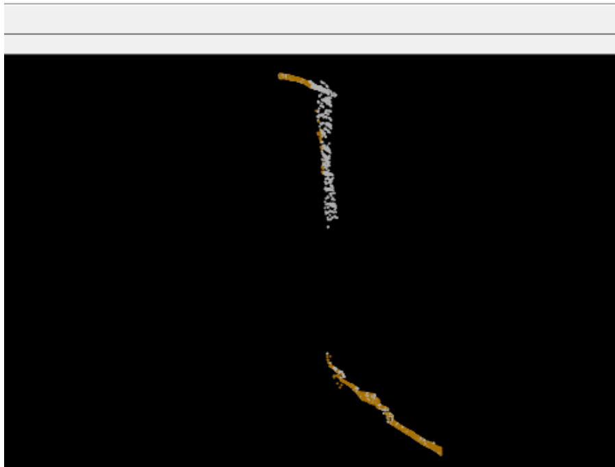
Figure 11. The image above shows an area of single swath coverage in the swath separation images and an LAS profile of the area. Due to the steep terrain, only one of the flightline coverages was able to acquire some returns along the near vertical cliff, even though at least two flightline coverages were acquired. Some of the terrain is so steep that no lidar returns are acquired along vertical portions of the terrain, regardless of the number of flightline coverages.
