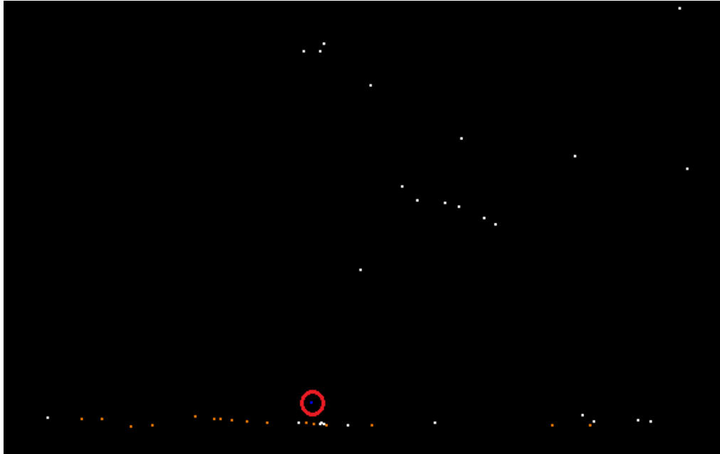
Figure 13-Checkpoint GWC 018 is shown as the blue dot circled in red. Overhead obstructions (white points) interfered with the collection of this checkpoint and it had to be removed from vertical accuracy testing.
