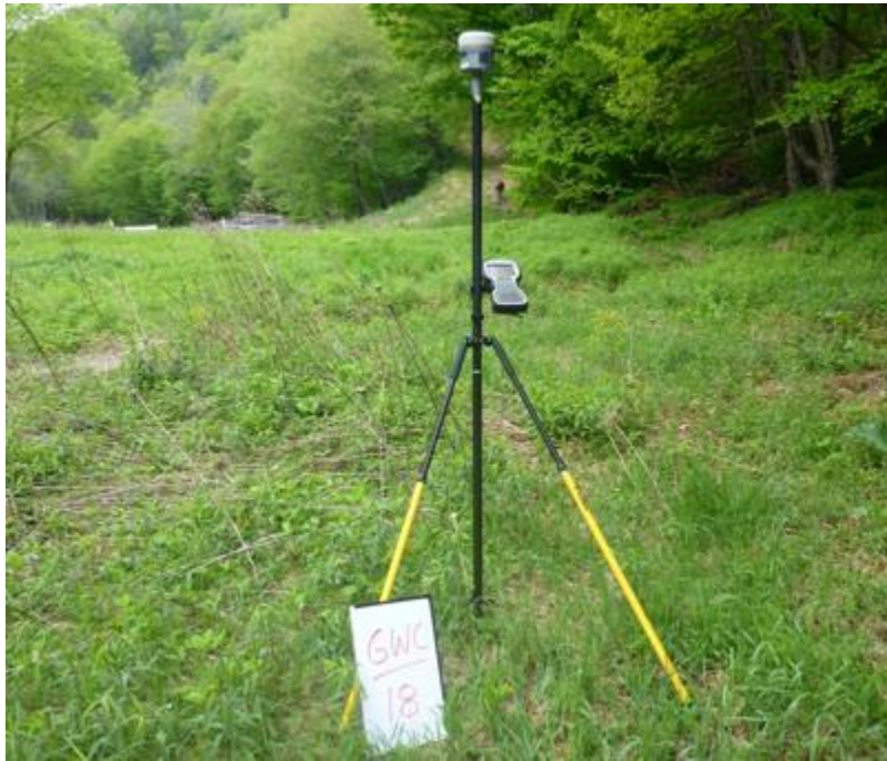
Figure 12-Checkpoint GWC 018. The surveyed elevation of this checkpoint is over 0.84 meters above the ground surface in the LiDAR data. Dewberry confirmed with the surveyors that overhead objects may have interfered with the GPS signals, resulting in an inaccurate elevation value for this checkpoint.
