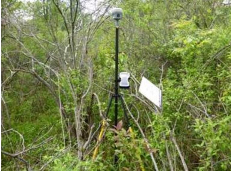
Figure 11-Checkpoint BLT 014. This survey checkpoint is located in extremely dense vegetation where light cannot reach the ground. Due to its poor location, this survey checkpoint was not used in vertical accuracy testing.
