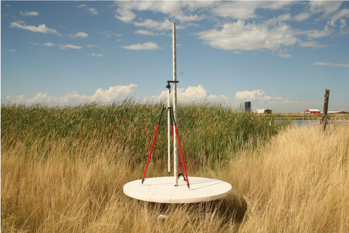
Figure 1. Example of lidar target along with equipment used to level its height relative to a nearby benchmark. This is benchmark 314RM in Davis County.
