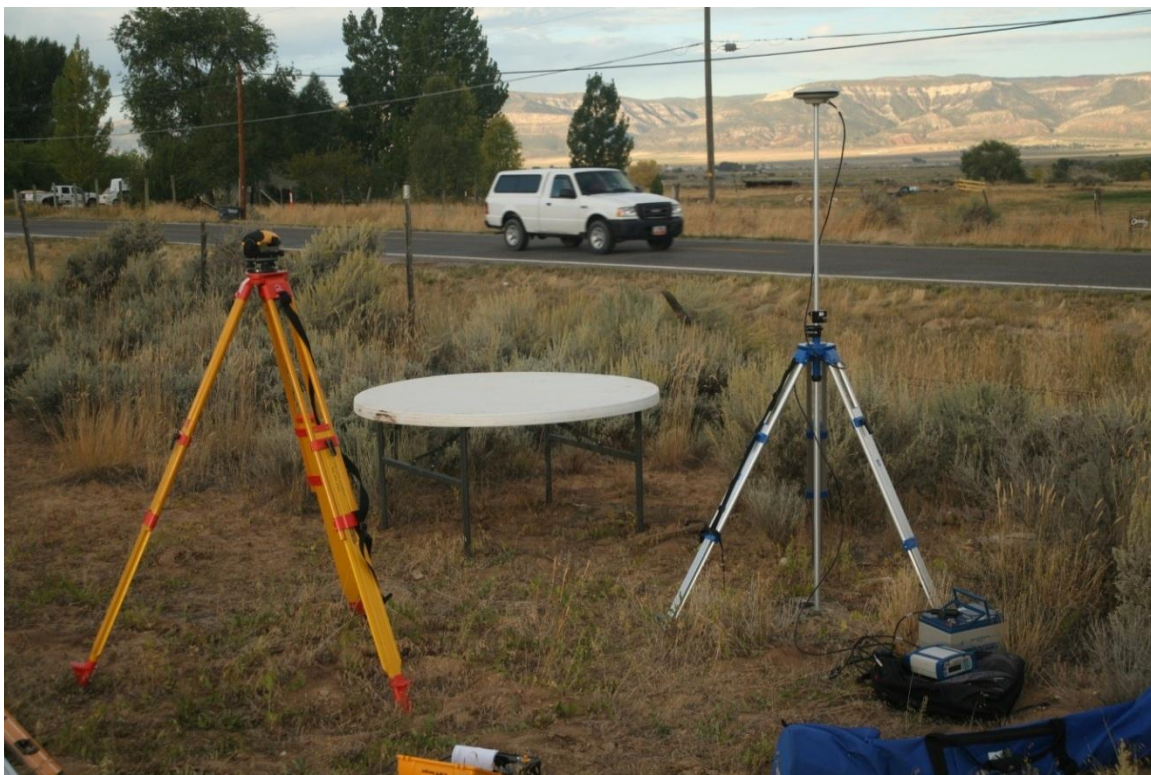
Figure 3. Lidar target next to NGS PID KN0377 “SPRING” monument occupied by the USU GNSS base station.
