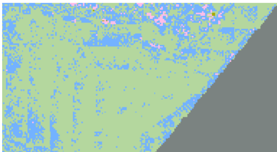
Figure 13 - Tile 17SQB530995- ( Green - < 0.0925m; Blue – 0.0925m to 0.18m; Pink – 0.18m to 0.36m, Grey- No Overlap) - Central Virginia Seismic data edge-matches with previously collected and accepted Louisa to create a seamless dataset. Some minor elevation differences exist in the bare-earth models between the two datasets, but 99% of measured differences are within the project specified RMSE z value of 0.0925 meters.
