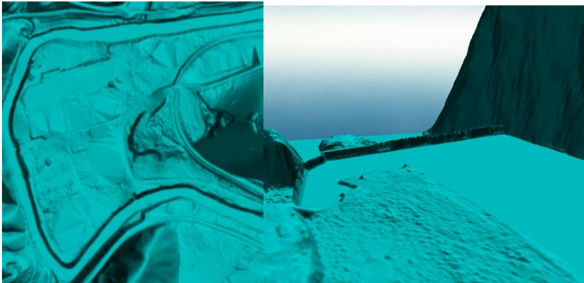
Figure 13- The image on the left shows a river segment that was hydro classified. These rivers were collected in areas that were below collection spec to maintain flow and to avoid sausage linking. The image on the right shows a dam that was left in the ground. The dam stops the flow of water and are to be left as ground.
