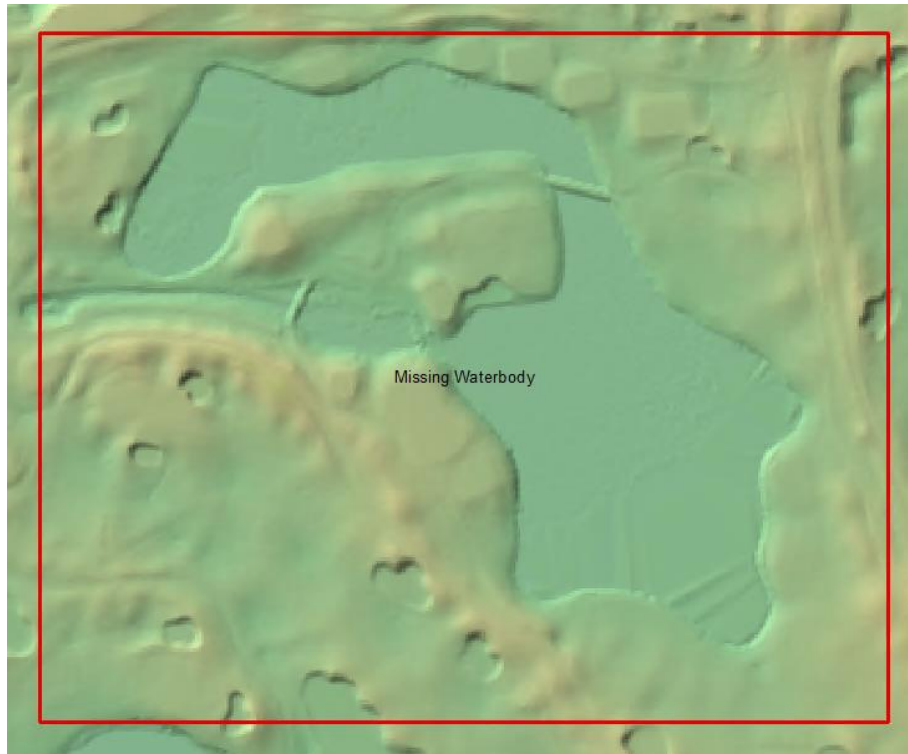
Figure 9 – Tiles e1588n1937 and e1588n1938. The image above is an overview of the DEM where USGS made a call stating that a waterbody larger than 2 acres was missing breaklines and was not hydroflattened.
