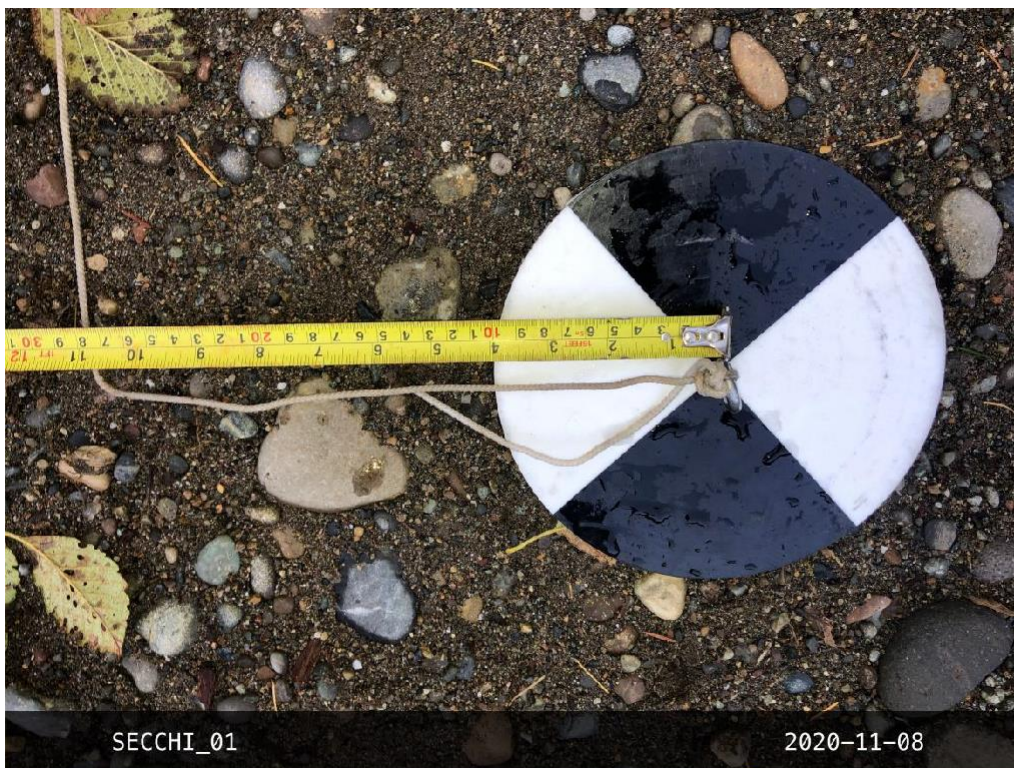
20 cm diameter, black and white secchi disk attached to rope
