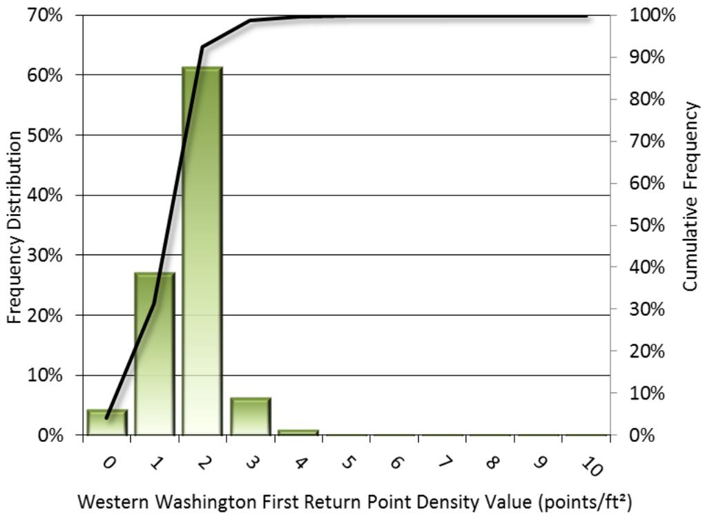
**Figure 6: Frequency distribution of first return point density values per 300 x 300 ft cell**
