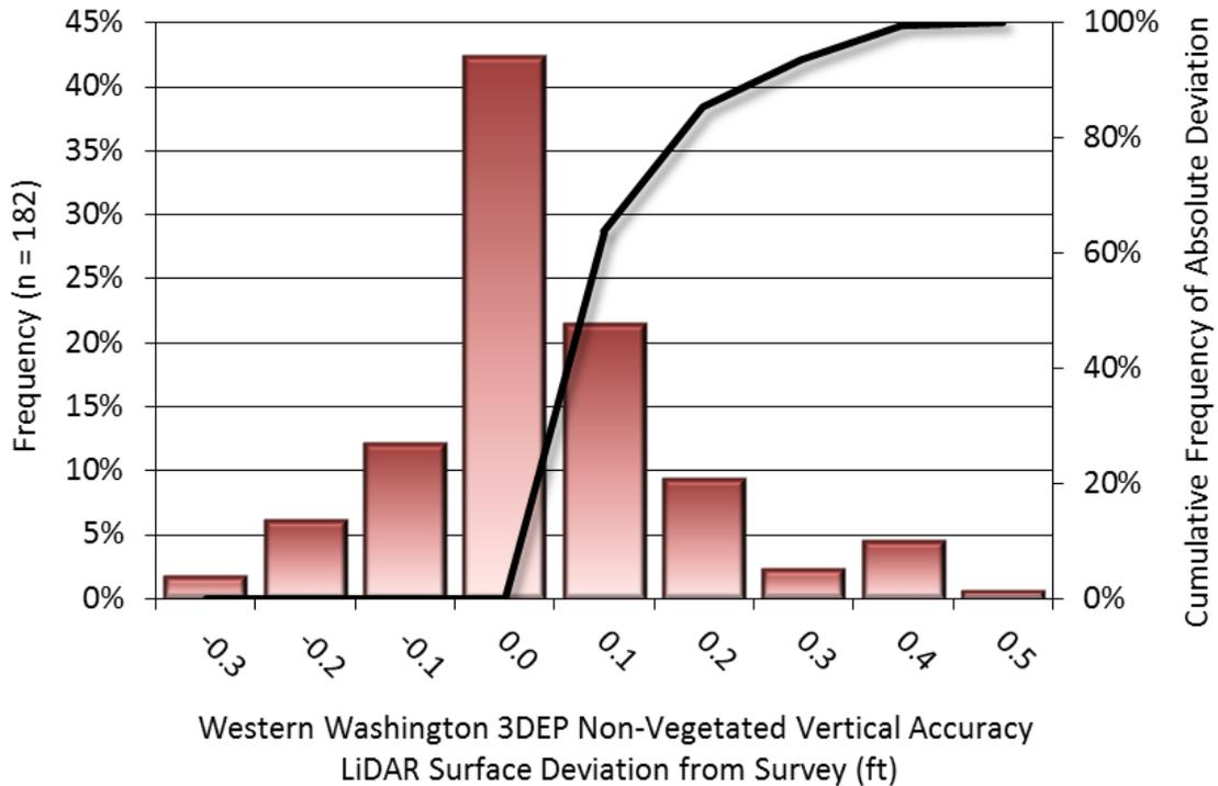
**Figure 8: Frequency histogram for LiDAR DEM surface deviation from non-vegetated quality assurance point values**
