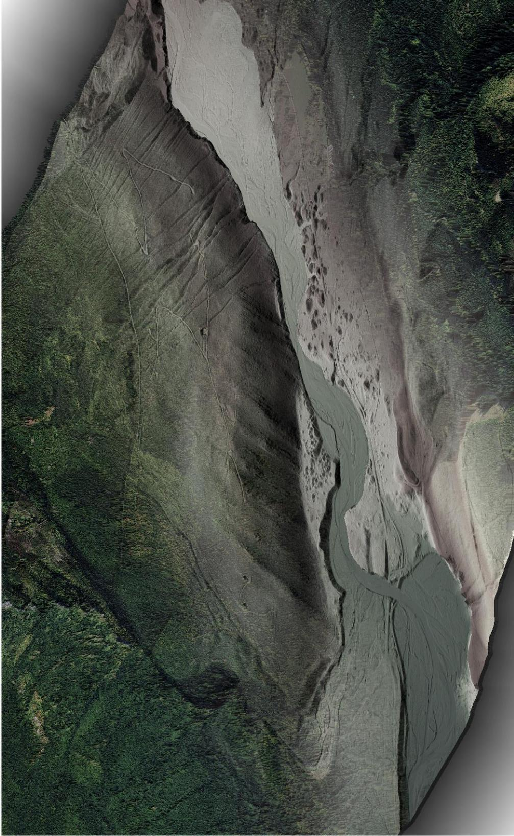
**Figure 14: This image shows a blended view of the Nooksack River and surrounding landscape, created from the bare earth DEM colored by elevation, partially overlaid with the above-ground point cloud colored using NAIP imagery.**
