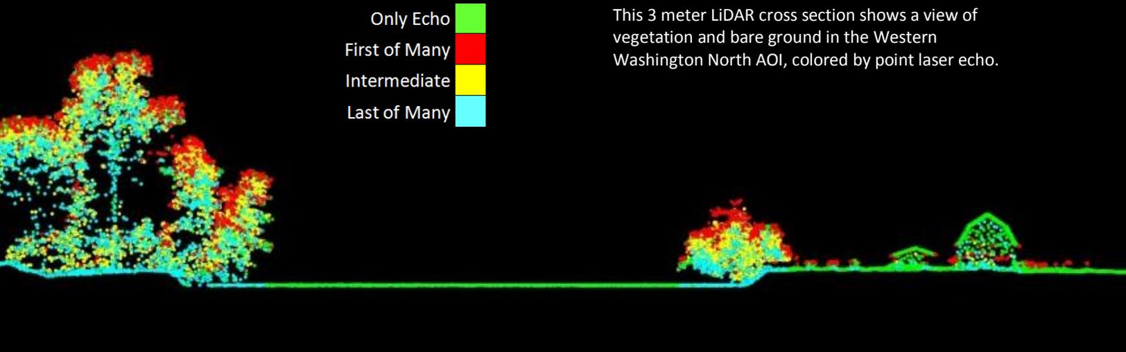
This 3 meter LiDAR cross section shows a view of vegetation and bare ground in the Western Washington North AOI, colored by point laser echo.
