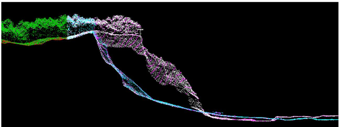
**Figure 5: This LiDAR cross section shows a view of a landslide which occurred along the Toutle River, and the temporal difference between the topography captured during LiDAR acquisition**
