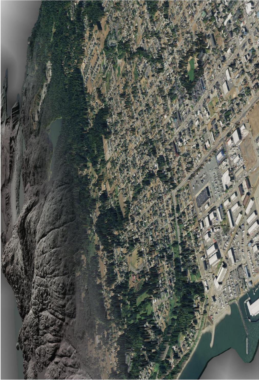
**Figure 13:** This image shows a view of Anacortes, Washington, created from the bare earth and above-ground point clouds colored by elevation and overlaid with NAIP imagery.
