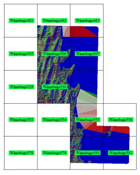
**QC Call:** Lake not hydro-flattened correctly (two features with two different elevations). (FID 4 in *Errors* shape file)
