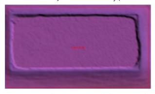
**QSI Response**: There was no water body present at the time of LIDAR collection. The points inside of the rectangular feature hold consistent elevation values, and there are no data voids delineating the possibility of a water body. There will be **no change** to this feature.
