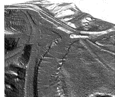
LiDAR surface before breaklines
