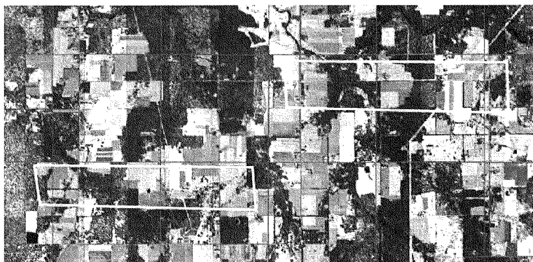
Swath to swath systematic errors are shown. TerraMatch uses the sample tiles to find biases between swaths and correct for them.
