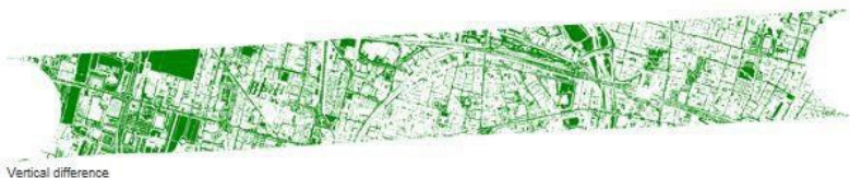
Figure 2 Vertical difference between forward and backward scan at 1000 m AGL.
