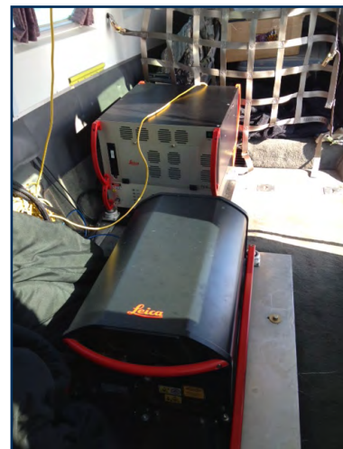
Above: Leica ALS70 mounted in the Navajo
