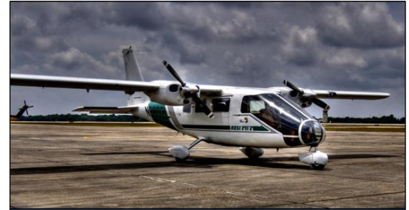
Above: A Partenavia P-68 is one platform for collecting LiDAR. Below: A Cessna Grand Caravan (208B) to gather orthophotos
