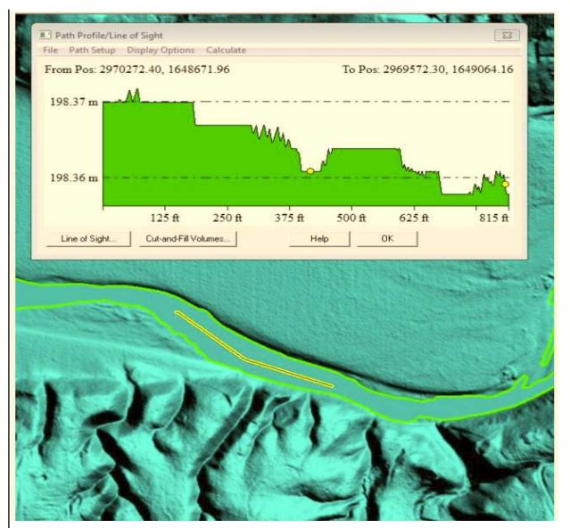
Hydroflattening of this stream/river is inconsistent. it is unclear why the hydroflattening process was completed up to this point then stopped
