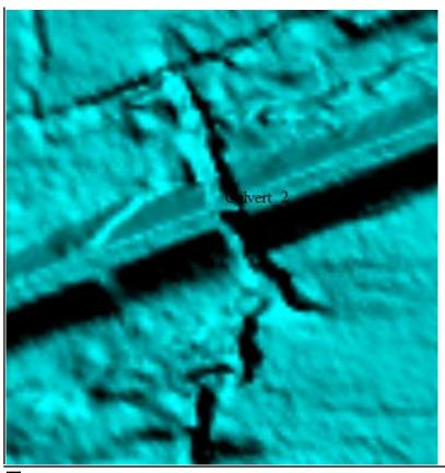
Depressions, Sinks, are not filled in (Not Hydro Conditioned)
