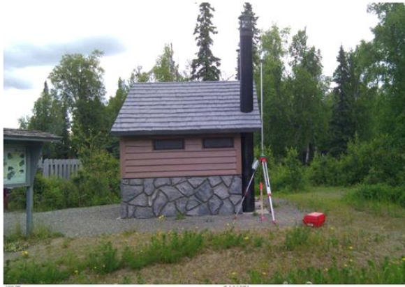
Figure 5, Checkpoint survey contractor pictures of CP 5-875 at corner of outhouse.
