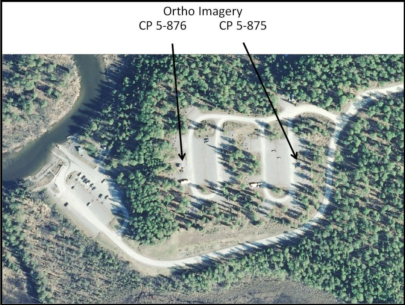
Figure 3, Ortho imagery with arrows pointing out two checkpoint locations in imagery.
