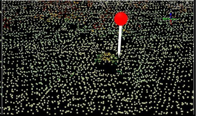
Figure 6, LiDAR point cloud assessment with QTM marking checkpoint location.
