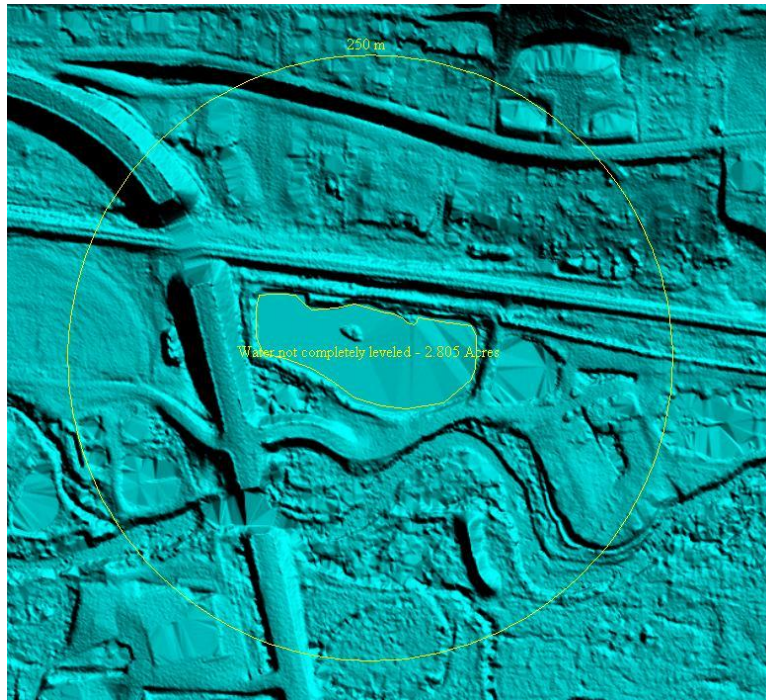
A. Original .img file: Water not leveled
