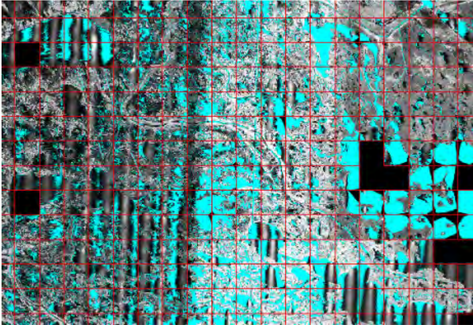
Figure 3 - Intensity images generated from full point cloud data. All areas that are bright blue indicate that there are no points in those areas because it is water. Large areas of water with no point returns will decrease the number of points per tile.
