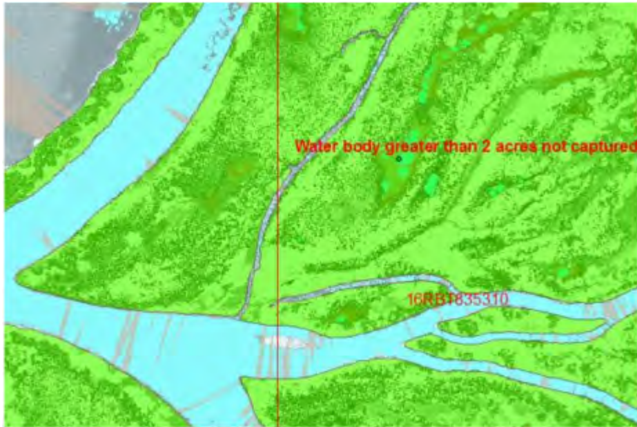
Figure 31 – 1 st delivery. Full point cloud intensity image with tidal waters (blue) and islands (green) draped over showing a water body that was not captured.
