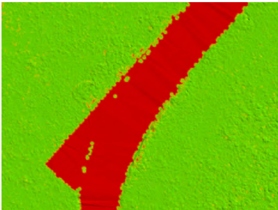
Figure 6 - Ground density model of Tile 15RXN615670 showing an area of ground (in red) that is currently unclassified (Class 1) and should be moved to ground (Class 2).
