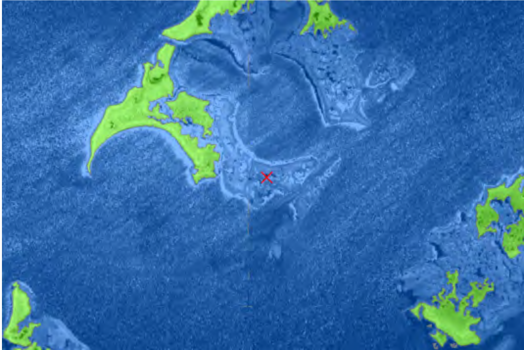
Figure 25- Tile 15RYN11265, first delivery. Island breaklines are colored transparent green, Tidal water breaklines are transparent blue. The LiDAR intensity image is visible underneath the breaklines. The image above shows ground that was captured as part of the tidal water breaklines.
