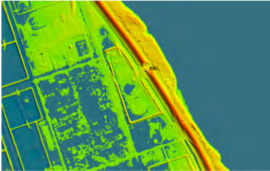
Figure 6 – 1 st delivery. Ground elevation model DEM of tile 16RBT115865 showing an area that is misclassified (move Class1-unclassified to Class 2-ground).
