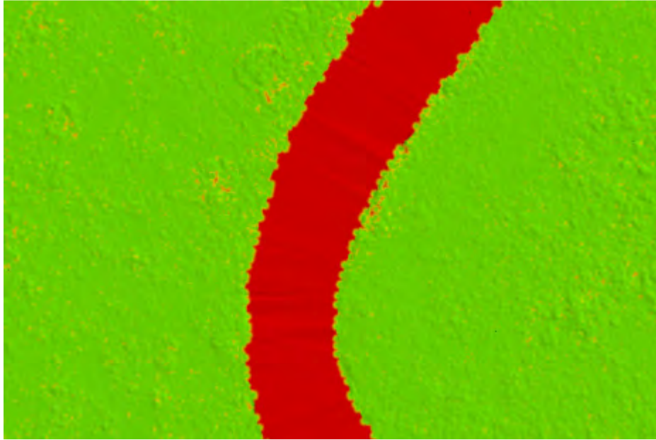
Figure 7 - Ground density model of Tile 15RXN615670 showing that the misclassification has been corrected in the second delivery.
