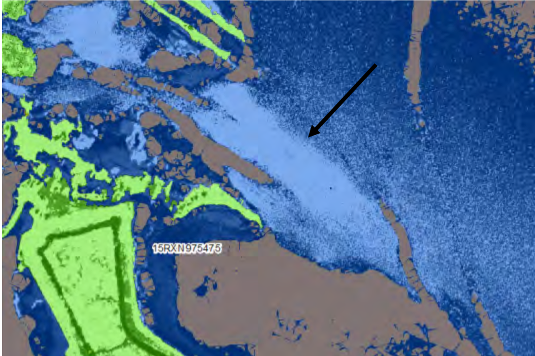
Figure 22 - Island breaklines are colored transparent green, Tidal water breaklines are transparent blue. The LiDAR intensity image is visible underneath the breaklines. Voids in the intensity image which represent water display in tan. The tidal water breaklines has been correctly adjusted to remove the issue.
