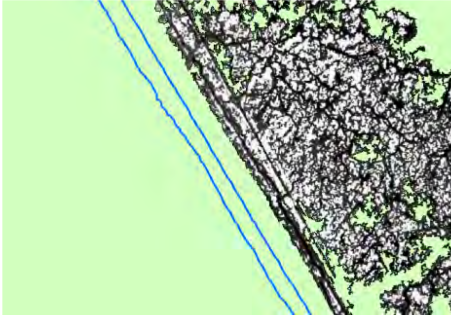
Figure 23 – 1 st delivery. Full point cloud intensity image of tile 16RBU190135. The green area is the islands breakline and the two blue lines delineate a stream breakline. The islands should be clipped at the stream lines.
