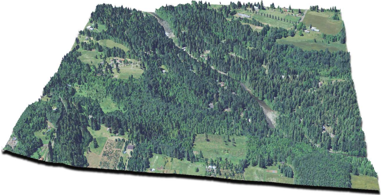
Figure 6.4: View upstream on the Sandy River over Revenue Bridge. Imagery created with RGB values extracted from 2009 NAIP orthophotos onto a three-dimensional point cloud.
