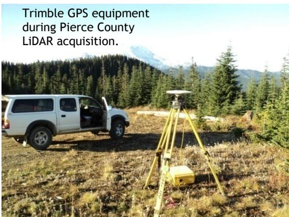
Trimble GPS equipment during Pierce County LiDAR acquisition.
