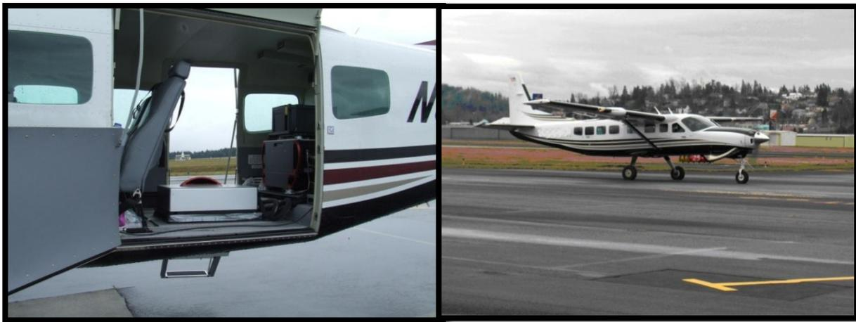
*The Cessna Caravan is a stable platform, ideal for flying slow and low for high density projects. The Leica ALS50 Phase II sensor head installed in the Caravan 208B is shown on the left.*
