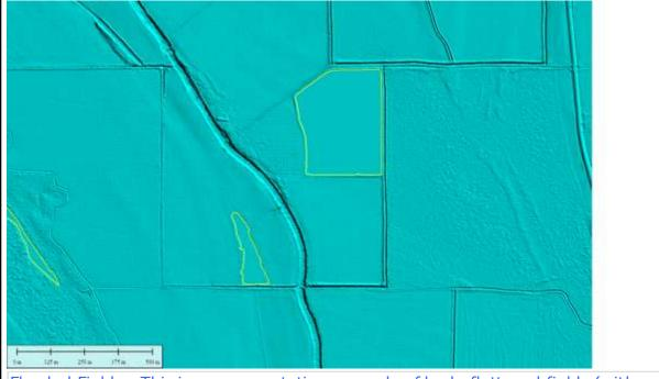
Flooded Fields: This is a representative example of hydroflattened fields (with breaklines); these occur throughout the project. These are not flagged as errors. The "flattened" fields suggest they were inundated at the time of lidar collection.
