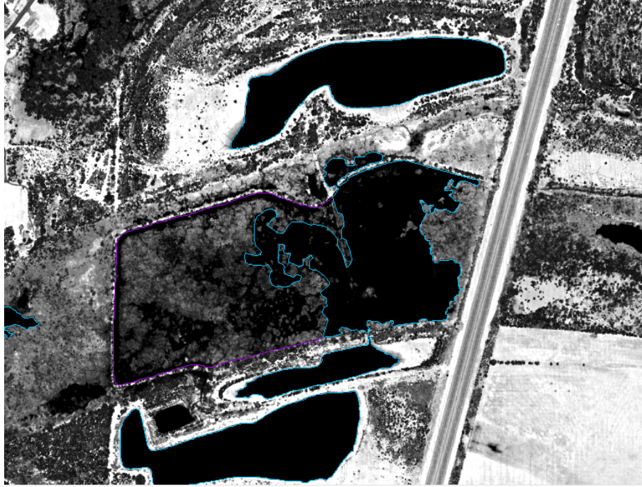
Figure 4: Tile 15WU2617. The intensity image showing the collected breaklines from the first delivery in purple and the modified breaklines from this delivery in blue.
