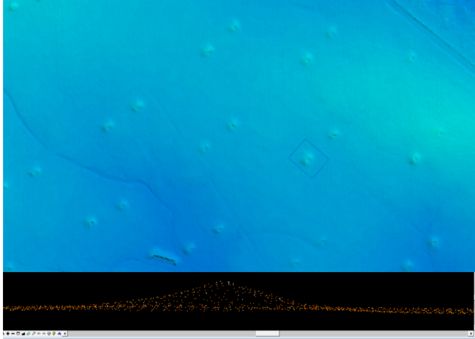
Figure 9 – Tile 15WU2220. The top view shows an elevation model of the area and the location of the profile. The bottom view shows a profile of the in ground structure where the unclassified points are white and the ground points are orange. The profile shows that the feature has correctly been left as ground.
