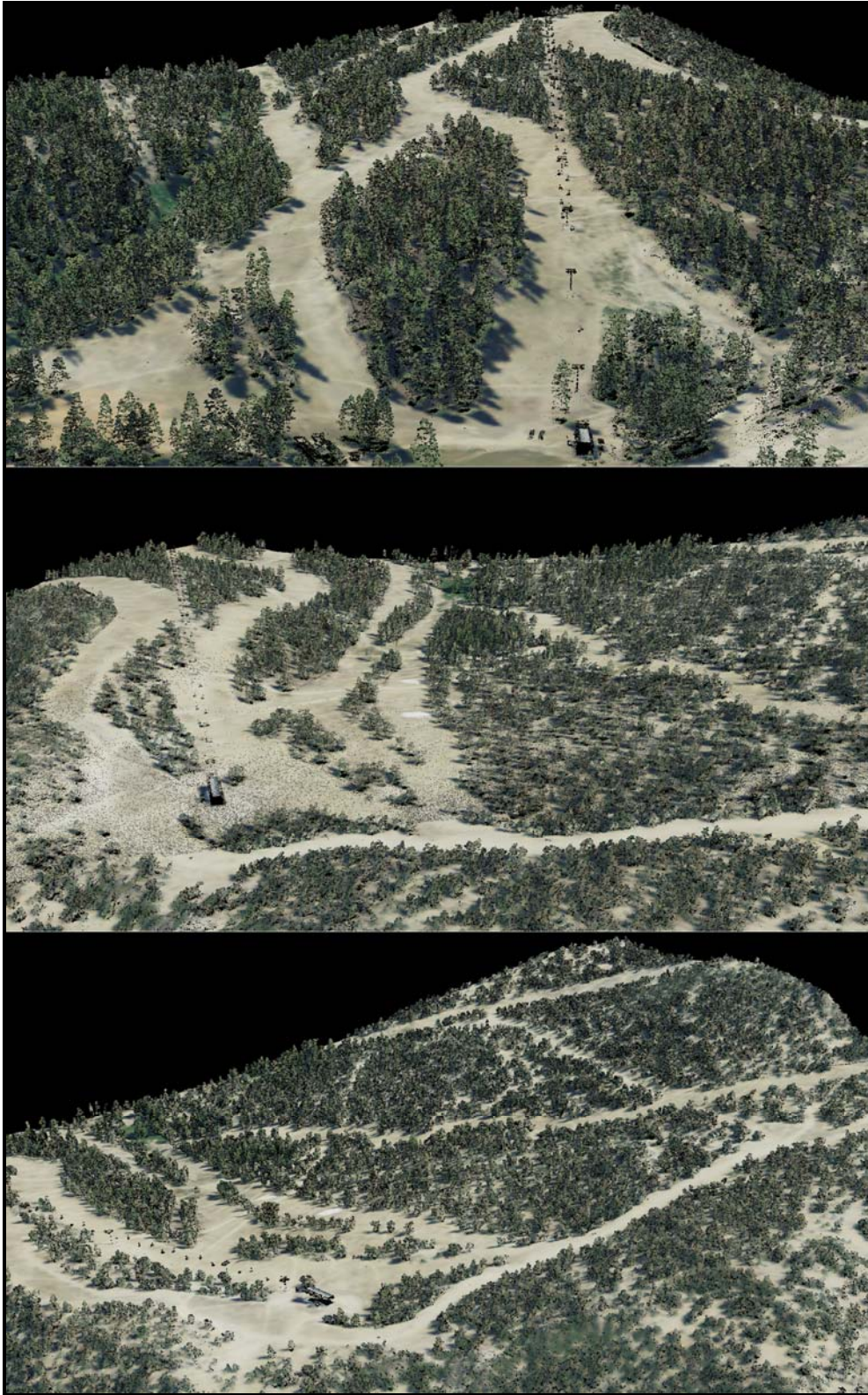
Figure 15. 3D LiDAR point cloud looking at Heavenly Ski Resort slopes (colored by 2009 NAIP)
