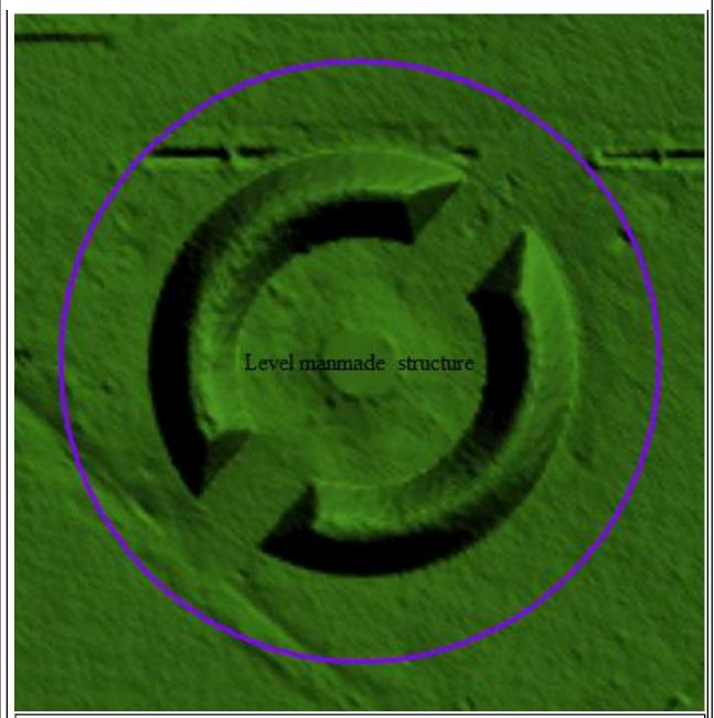
Reviewer identified a man-made structure in bare earth surface. This error is documented in a shapefile created by the reviewer at NGTOC named errors.shp. In the pdf, "Dewberry Response to USGS Review Orange County 10012012" Dewberry explains that in this instance earthen mounds have been formed around the feature and have been correctly included in the ground classification. Reviewer accepts this response.
