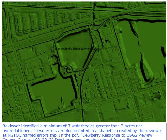
Orange County 10012012" Dewberry explains that one of four calls regarding breaklines/waterbodies was incorrect, from viewing the intensity images it can be determined that no water existed at the time of acquisition. The other three calls were addressed, corrected, and new DEM and LAS files were redelivered to the reviewer via ftp site on 10/02/12. Reviewer visually inspected the redelivered DEMs and found them acceptable.
