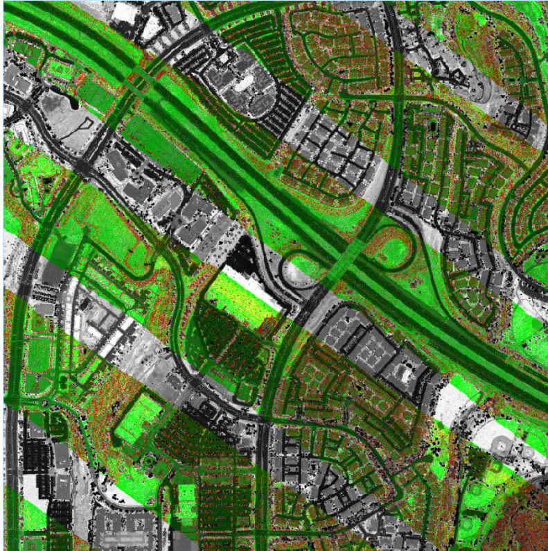
Figure 3: DZ orthos created from the full point cloud. Some red pixels are visible along embankments, sloped terrain, and in vegetated land cover, as expected. Open, flat areas are green indicating the calibration and relative accuracy of the data is acceptable.
