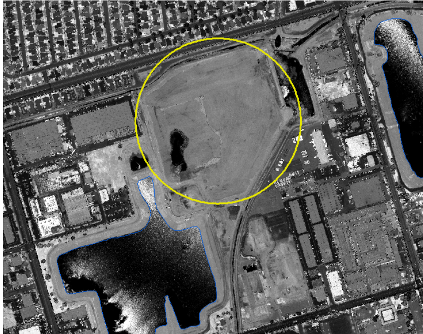
Figure 19 - Tile 11SMT201465. As the intensity imagery shows, the breaklines delivered to USGS correctly capture the water bodies in the area that are 2 acres or greater.
