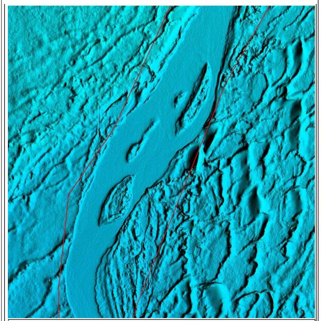
\*Determined this is acceptable. Above is a DLS which has a greater than 100ft nominal width (near the sand dunes), but was not flattened. As with many of the retention ponds and waterbodies, it exhibits higher point density and little tinning indication dry or shallow conditions and need not be flattened.
