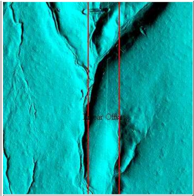
Linear offsets such as the one pictured are rare in the dataset and do not significantly effect the elevations in the DEM. Moreover, it is not clear if this is caused by a genuine calibration/registration issue, natural fault, or software visualization, but the events have been noted and tagged.
