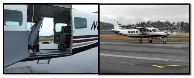
The Cessna Caravan is a stable platform, ideal for flying slow and low for high density projects. A Leica ALS50ii sensor head installed in the Caravan is shown on the left.
