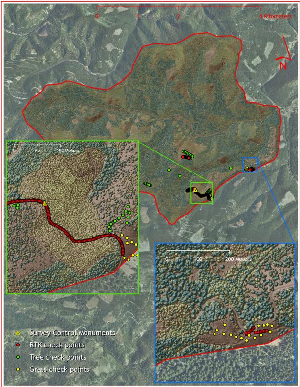
Figure 8. RTK check point, land cover check points, and control monument locations used in the Deception AOI.
