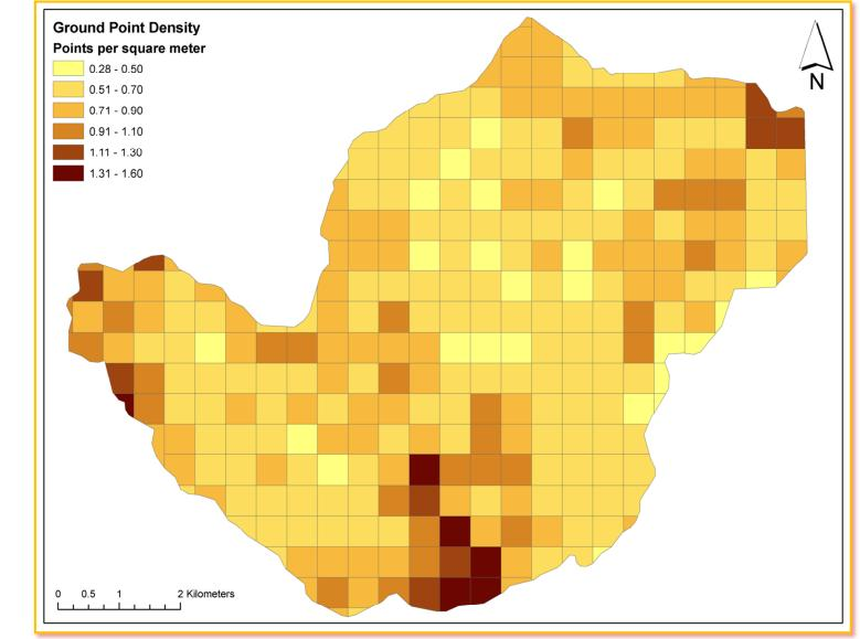
Figure 12. Density distribution map for ground return points by processing bin for Laundry China Osier AOI
