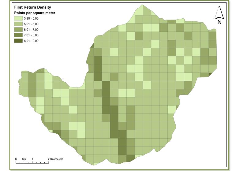
Figure 11. Density distribution map for first return points by processing bin for Laundry China Osier AOI
