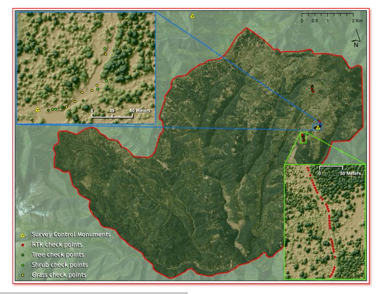
Figure 2. RTK check points, land cover check points, and control monument locations used in the Laundry China Osier AOI.
