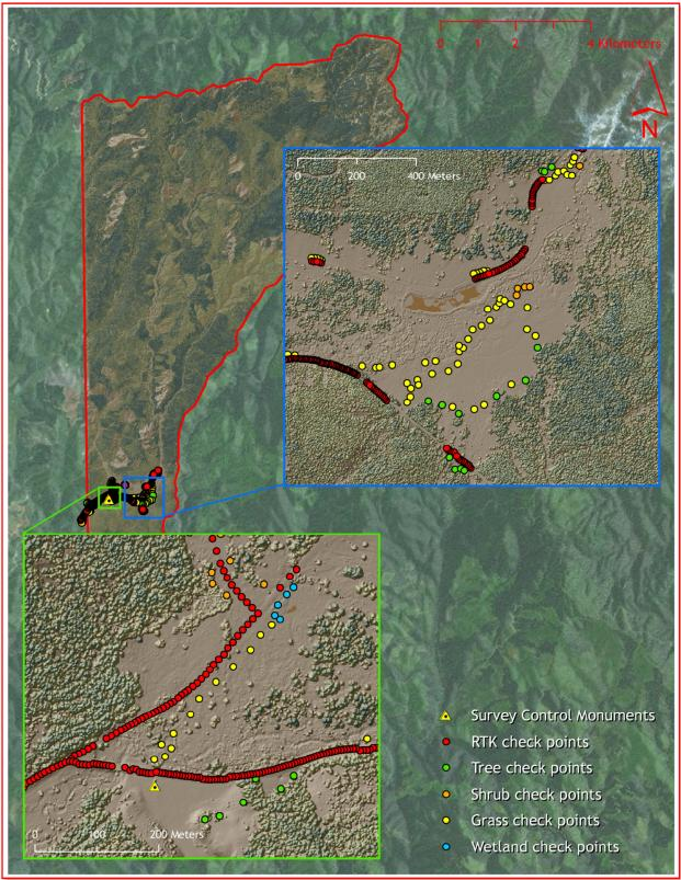
*Figure 6.* RTK check point, land cover check points, and control monument locations used in the Musselshell AOI.
