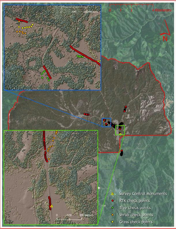
*Figure 5. RTK* check point, land cover check points, and control monument locations used in the Potlatch AOI.
