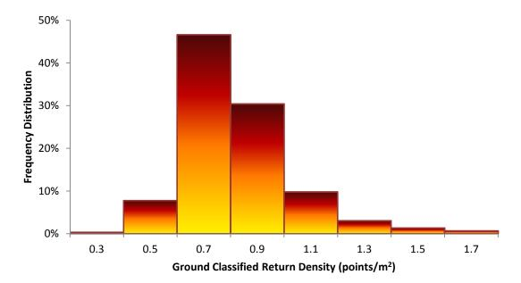
Figure 10. Density distribution for ground classified laser points
