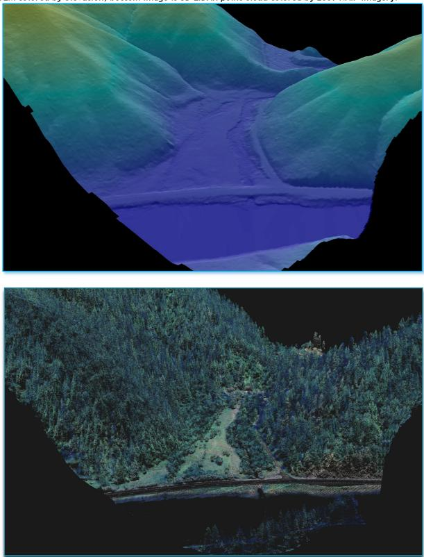
**Figure 48**. Intersection of Pete King Road and Hwy 12, looking northwest. Top image is bare earth DEM colored by elevation, bottom image is 3D LiDAR point cloud colored by 2009 NAIP imagery.
