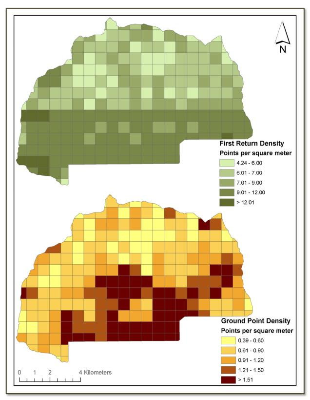
Figure 29. Density distribution map for first return points by processing bin for the Potlatch AOI
