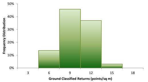
Figure 28. Density distribution for ground classified laser points
