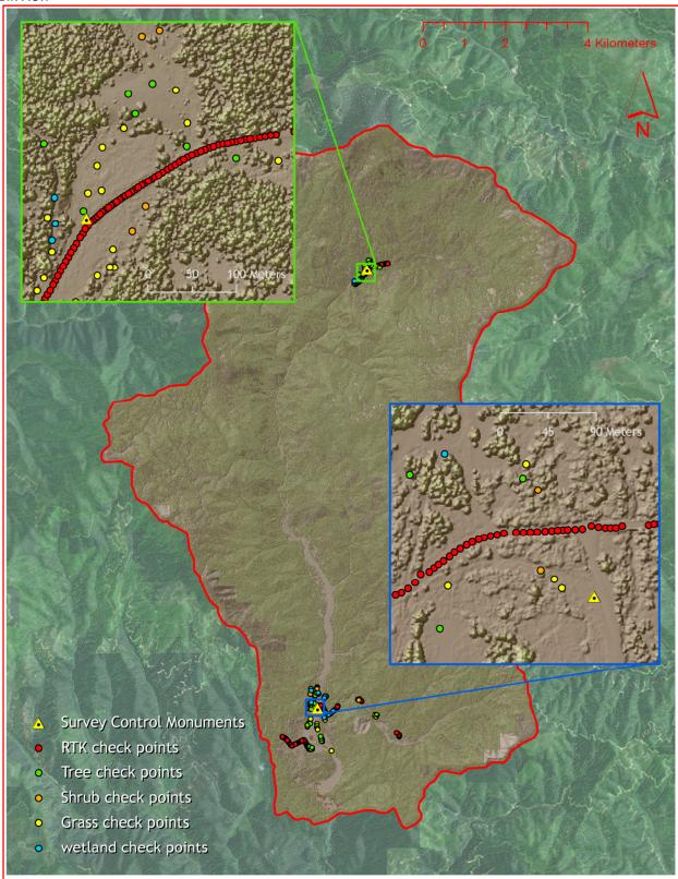
*Figure 4.* RTK check point, land cover check points, and control monument locations used in the Upper *Elk AOI*.
