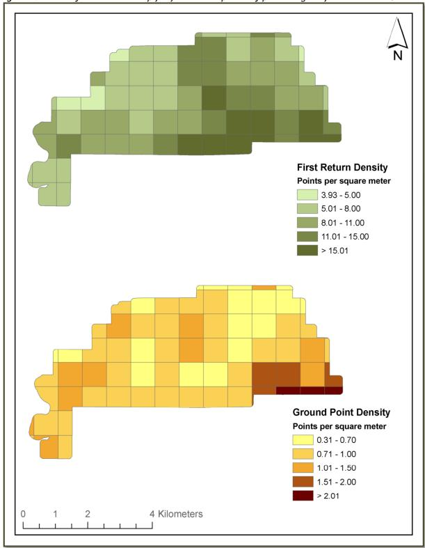
Figure 39. Density distribution map for first return points by processing bin for the Priest AOI
