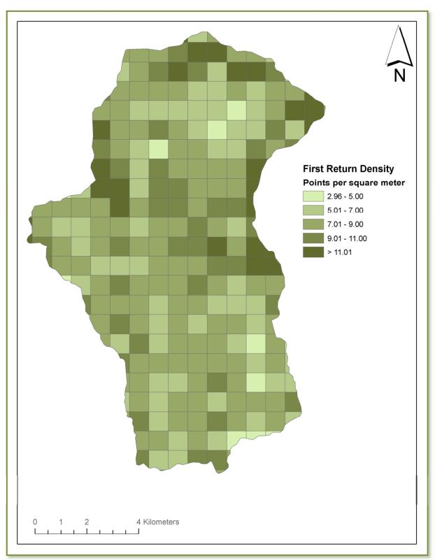
Figure 23. Density distribution map for first return points by processing bin for the Upper Elk AOI
