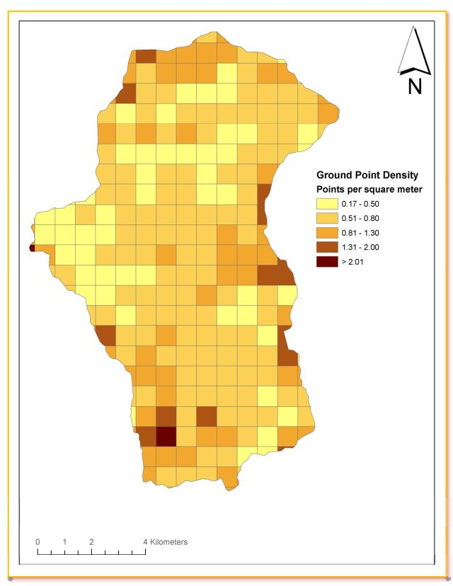
Figure 24. Density distribution map for ground return points by processing bin for the Upper Elk AOI
