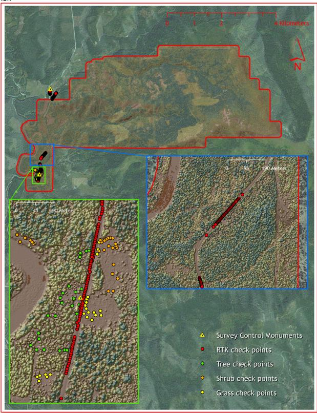
*Figure 7. RTK* check point, land cover check points, and control monument locations used in the Priest AOI.
