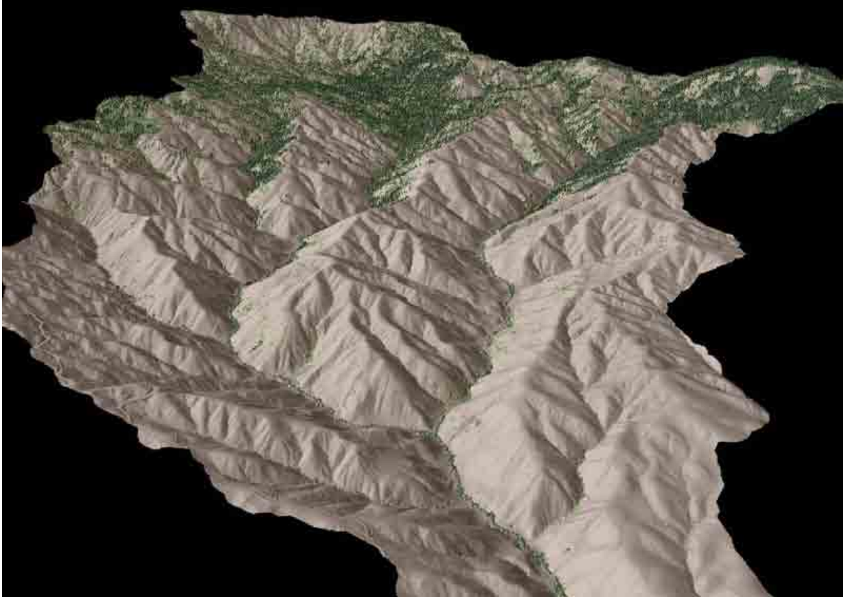
Figure 20. Oblique view of Boise Front AOI: Above Ground ESRI Grid (1-meter resolution) derived from all LiDAR points
