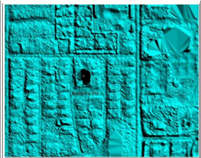
A low point was created in bare earth surface when building removed. Reviewer created a shapefile showing location of errors in the delivered DEMs. Shapefile is named DEM\_Errors\_BartholomewCo and is located in the NED\Errors folder. Scale as shown is approximately 1:3947. Corrections completed at NGTOC, accepted 11/18/13.
