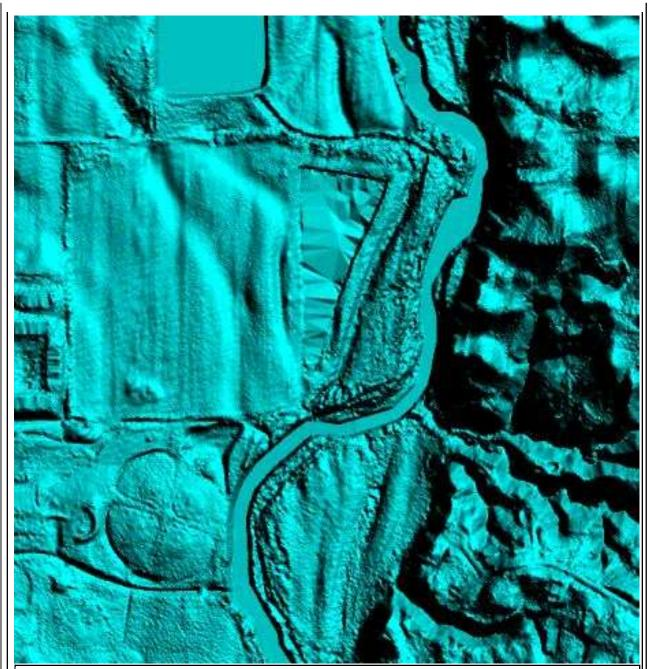
Waterbodies larger than 2 acres need to be hydro flattened. Reviewer created a shapefile showing location of errors in the delivered DEMs. Shapefile is named DEM\_Errors\_BartholomewCo and is located in the NED\Errors folder. Scale as shown is approximately 1:8743. Corrections completed at NGTOC, accepted 11/18/13.
