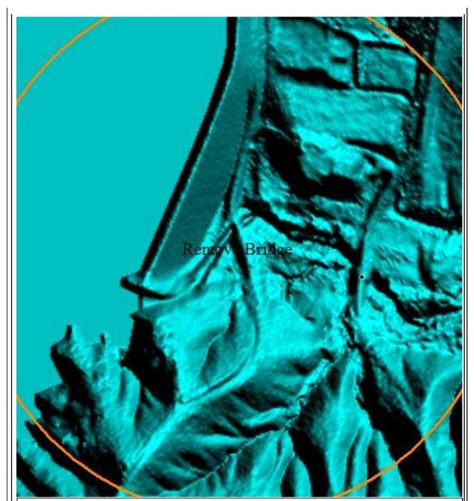
Bridges need to be removed from bare earth surface. Reviewer created a shapefile showing location of errors in the delivered DEMs. Shapefile is named DEM\_Errors\_BartholomewCo and is located in the NED\Errors folder. Scale as shown is approximately 1:3461. Corrections completed at NGTOC, accepted 11/18/13.
