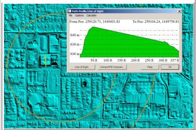
Building not completely removed. Reviewer created a shapefile showing location of errors in the delivered DEMs. Shapefile is named DEM\_Errors\_BartholomewCo and is located in the NED\Errors folder. Scale as shown is approximately 1:12390. Corrections completed at NGTOC, accepted 11/18/13.
