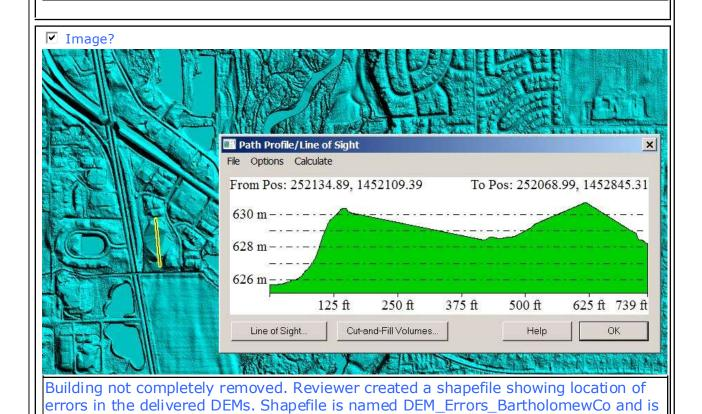
located in the NED\Errors folder. Scale as shown is approximately 1:16540. Corrections completed at NGTOC, accepted 11/18/13.
