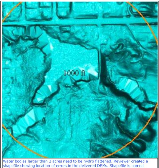
shapefile showing location of errors in the delivered DEMs. Shapefile is named DEM\_Errors\_BooneCo and is located in the NED\Errors folder. Scale as shown is approximately 1:6500. Radius of circle in shapefile is 1000 feet. DEM cell is in2011\_31701710\_12. Corrections performed in house, accepted 12/12/13.
