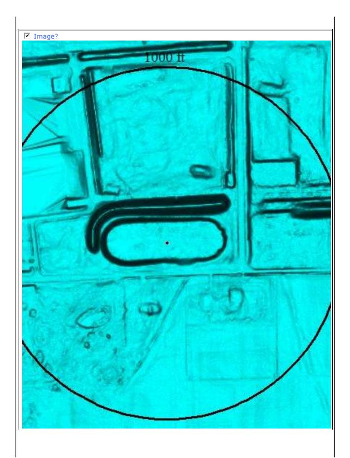
Water bodies larger than 2 acres need to be hydro flattened. Reviewer created a shapefile showing location of errors in the delivered DEMs. Shapefile is named DEM\_Errors\_BooneCo and is located in the NED\Errors folder. Scale as shown is approximately 1:6000. Radius of circle in shapefile is 1000 feet. DEM cell is in2011\_31501720\_12. Corrections performed in house, accepted 12/12/2013.
