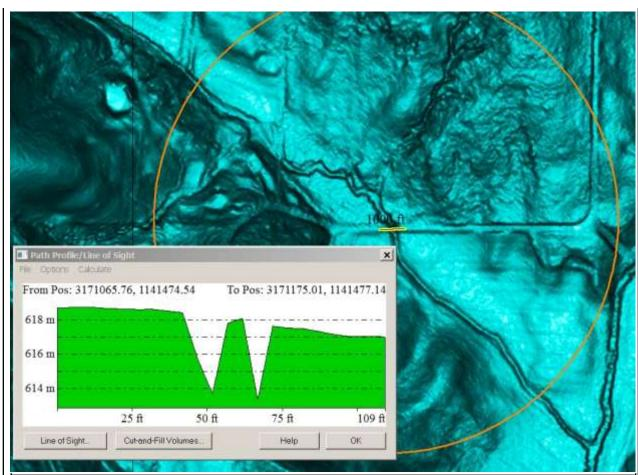
Bridges need to be completely removed. If imagery does not support presence of a bridge then culvert should be assumed and consistency of road fill reflected in DEM. Reviewer created a shapefile showing location of errors in the delivered DEMs. Shapefile is named DEM\_Errors\_CrawfordCo and is located in the NED\Errors folder. Radius of circle in shapefile is 1000 feet. DEM cell is in2011\_31701140\_12. Corrections performed at NGTOC, accepted 12/13/13.
