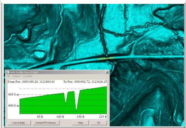
Bridges need to be completely removed. If imagery does not support presence of a bridge then culvert should be assumed and consistency of road fill reflected in DEM. Reviewer created a shapefile showing location of errors in the delivered DEMs. Shapefile is named DEM\_Errors\_CrawfordCo and is located in the NED\Errors folder. Radius of circle in shapefile is 1000 feet. DEM cell is in2011\_30901120\_12. Corrections performed at NGTOC, accepted 12/13/13.
