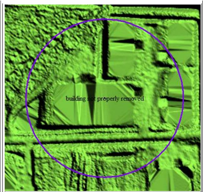
Building not properly removed. Reviewer created a shapefile documenting the location of errors found in the delivered DEMs named errors.shp which is located in the NED-Errors folder. On 8/8/13 reviewer was notified that no corrections will be delivered to NGTOC. Corrections performed in house, accepted 12/13/13.
