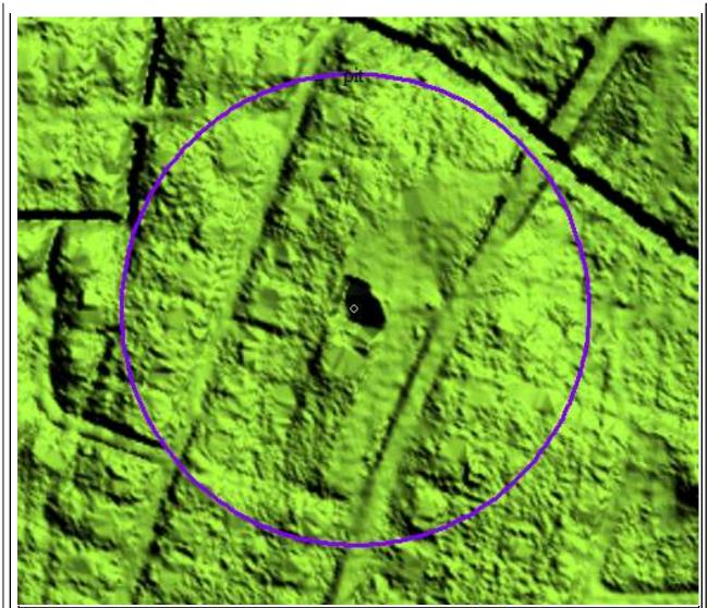
Pit found in bare earth surface. Reviewer created a shapefile documenting the location of errors found in the delivered DEMs named errors.shp which is located in the NED-Errors folder. On 8/8/13 reviewer was notified that no corrections will be delivered to NGTOC. Corrections performed in house, accepted 12/13/13.
