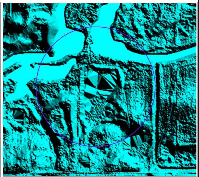
One waterbody greater than 2 acres that was not hydroflattened was identified by the reviewer. This is the only error that requires correction. It is located in DEM tile in2011\_02051905\_12.img. Reviewer created a shapefile documenting the location of this error found in the delivered DEMs named errors.shp. On 8/8/13 reviewer was notified that no corrections will be delivered to NGTOC. Corrections performed in house, accepted 11/19/13.
