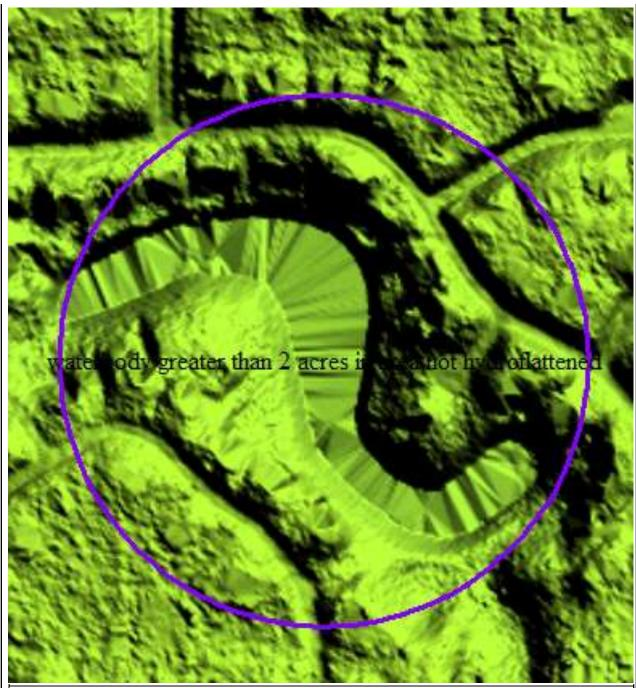
Waterbody greater than 2 acres in area not hydroflattened. Reviewer created a shapefile documenting the location of errors found in the delivered DEMs named errors.shp which is located in the NED-Errors folder. On 8/8/13 reviewer was notified that no corrections will be delivered to NGTOC. Corrections performed at NGTOC, accepted 12/16/13.
