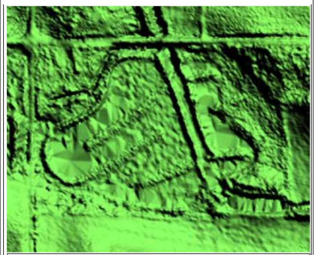
Waterbody greater than 2 acres in area not hydroflattened. Observed scale 1:6000. Reviewer created a shapefile documenting the location of errors found in the delivered DEMs named errors.shp which is located in the NED-Errors folder. On 8/8/13 reviewer was notified that no corrections will be delivered to NGTOC. Corrections performed at NGTOC, accepted 12/19/13.
