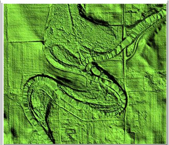
Double line stream greater than 100 feet not hydro-enforced. Observed scale 1:6000. Reviewer created a shapefile documenting the location of errors found in the delivered DEMs named errors.shp which is located in the NED-Errors folder. On 8/8/13 reviewer was notified that no corrections will be delivered to NGTOC. Corrections performed at NGTOC, accepted 12/19/13.
