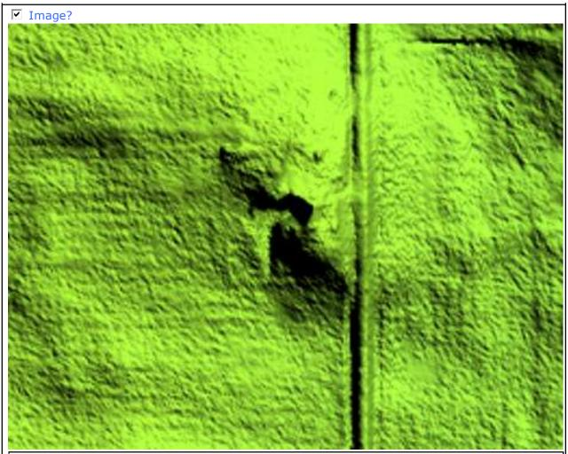
Low point resulting in a pit left in bare earth surface. Observed scale 1:3186. Reviewer created a shapefile documenting the location of errors found in the delivered DEMs named errors.shp which is located in the NED-Errors folder. On 8/8/13 reviewer was notified that no corrections will be delivered to NGTOC. Corrections performed at NGTOC, accepted 12/19/13.
