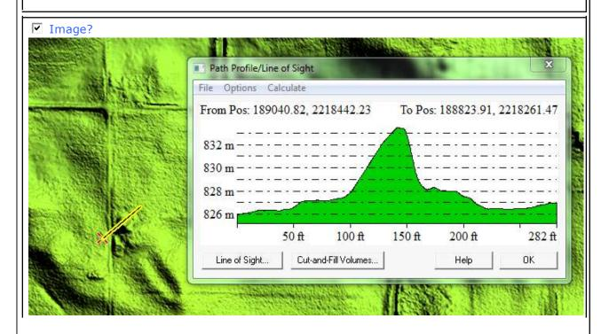
Building not removed from bare earth surface. Observed scale 1:5206. Reviewer created a shapefile documenting the location of errors found in the delivered DEMs named errors.shp which is located in the NED-Errors folder. On 8/8/13 reviewer was notified that no corrections will be delivered to NGTOC. Corrections performed at NGTOC, accepted 12/19/13.
