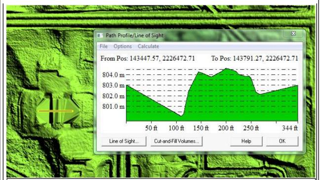
Building not properly removed. Observed scale 1:5142. Reviewer created a shapefile documenting the location of errors found in the delivered DEMs named errors.shp which is located in the NED-Errors folder. On 8/8/13 reviewer was notified that no corrections will be delivered to NGTOC. Corrections performed at NGTOC, accepted 12/19/13.
