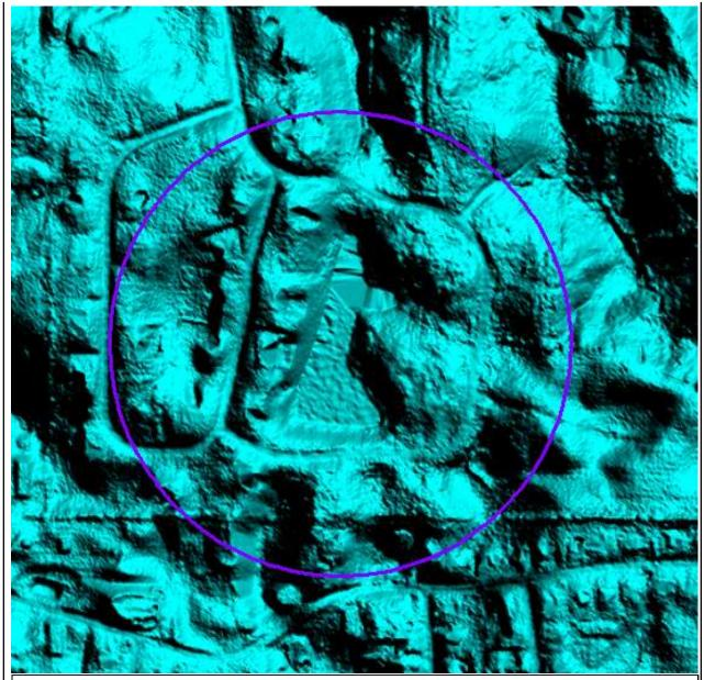
Waterbody greater than 2 acres in area not hydroflattened. This is unacceptable as USGS Base Spec v12 explicitly requires hydroflattening of waterbodies greater than 2 acres in area. Reviewer created a shapefile documenting the location of errors found in the delivered DEMs named errors.shp which is located in the NED-Errors folder. On 8/8/13 reviewer was notified that no corrections will be delivered to NGTOC. Multiple corrections performed at NGTOC, accepted 12/5/13.
