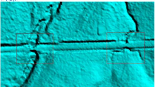
As with Harvey Co., several errors exist in dataset in which culverts were removed completely or partially as seen above when they should be left in data. This is a representative image of the errors. Only a few of this type of error were called due to it being endemic throughout. Location at 38° 05' 8.1436" N, 96° 49' 17.6969" W
