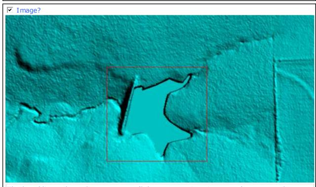
The breaklines along the waterways (lakes, reservoirs, rivers, etc) appear to be deeper than they actually are (look very steep-sided). This location is at  $38^{\circ}$  51' 57.4955" N,  $96^{\circ}$  42' 59.6017" W
