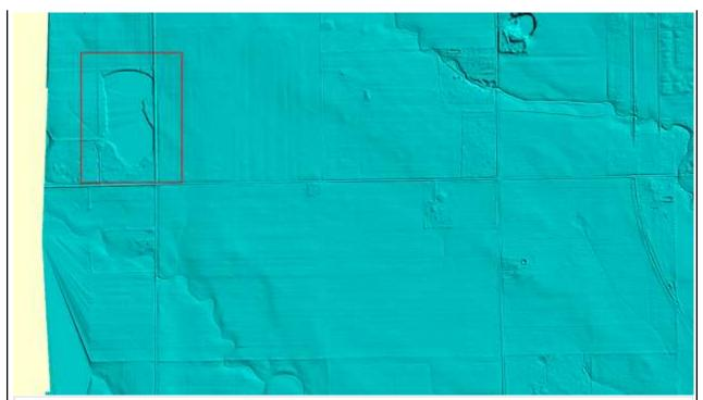
Lake not hydroflattened. There are two errors of this type. Location at 38° 00' 57.7723" N, 97° 42' 9.6131" W
