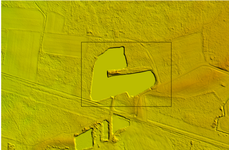
Figure 10 - Tiles 18SVH299583, 18SVH314583, 18SVH299568, and 18SVH314568. An additional pond breakline has been collected for this feature and used to flatten the feature in the redelivered DEM. The LAS have been corrected to reflect the addition of this feature.
