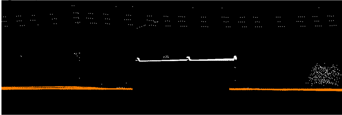
Figure 3-Tile 18SVH479493. No additional points can be removed from ground classification. Bridge “saddles” are a visual artifact resulting from interpolation of a continuous surface.
