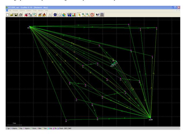
The survey was controlled against three provided control points M15, M302 and M303. These points were checked against CORS site BLMN and MOSL.
